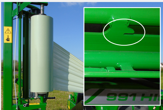
Lower dispenser threading path
