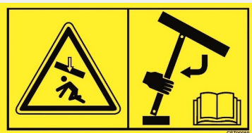
Support table before working under it Refer to the instruction manual (CST00059)
