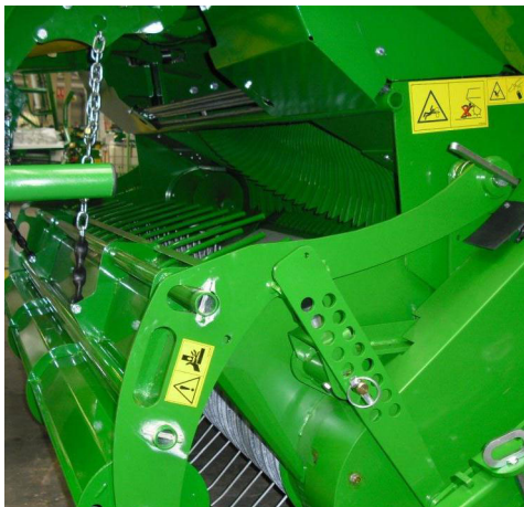
Crop roller adjustment chain
