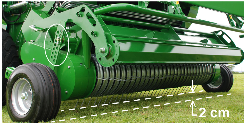
Pick-up reel height adjustment
