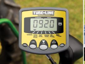
The wrap counter allows you to set the desired number of rotations of wrap per bale and displays the current rotation.
