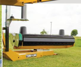
Located on the turntable, the two rollers spin the bale while wrapping, ensuring it's completely sealed.
