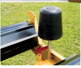
Adjustable bale guides allow 4' or 5' bales to be centered on the turntable ensuring even delivery of wrap.
