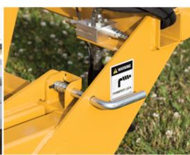
The manual transport lock secures the bale platform to prevent dumping during transport.
