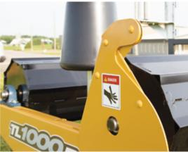
After a bale has been unloaded and a new one is placed on the turntable, the knife easily cuts the plastic wrap for continuous operation.
